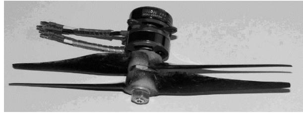
Gambar 9. *Contra rotating propeller* [8]
