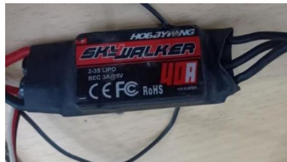
**Gambar 3.** *Electronic speed controller*
